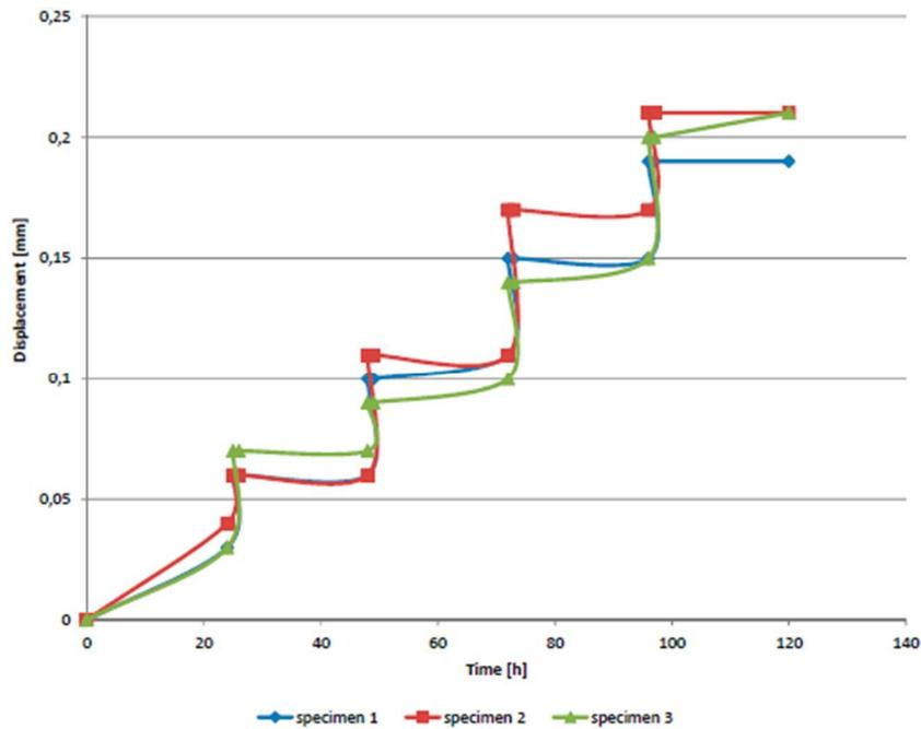
**Figure 1: Deflection curve in function of time**
